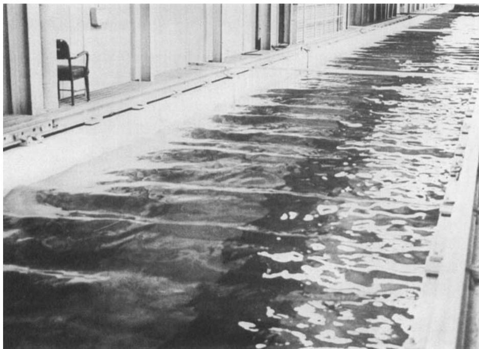
FIGURE 6. Two-dimensional wave forms after disappearance of spilling breakers.
