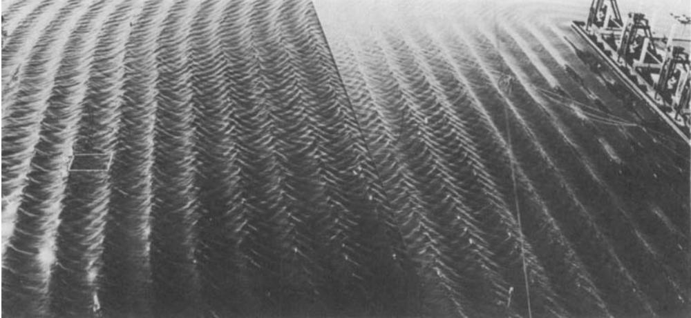
FIGURE 14. The wavemaker and the wave patterns in the wave basin up to  $x = 15.5$  m with  $f_0 \approx 1.55$  Hz,  $(ak)_0 = 0.32$ . Picture is taken from a tower at 12 m above mean water surface. The expansion angle is  $\theta \approx 17^\circ$ .
