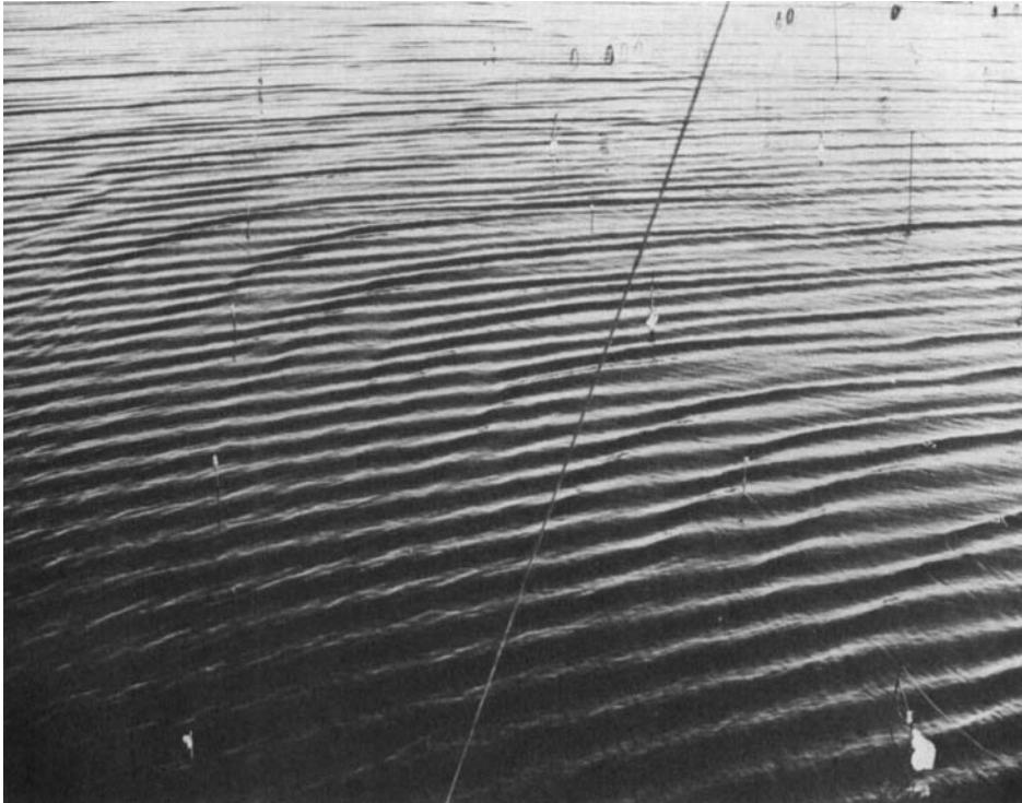
FIGURE 19. Wave patterns at the final stage of the evolution starting in figure 14. The oblique wave groups due to three-dimensional wave breaking are propagating from the lower right corner to the upper left corner of the photograph.
