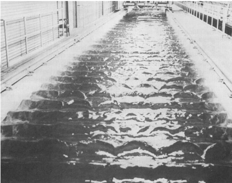
FIGURE 4. Three-dimensional spilling breakers at  $x \approx 18$  m to  $x \approx 25$  m.
